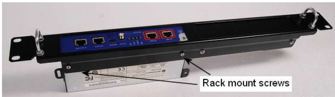
Figure 109 PTP-SYNC mounted in a rack
