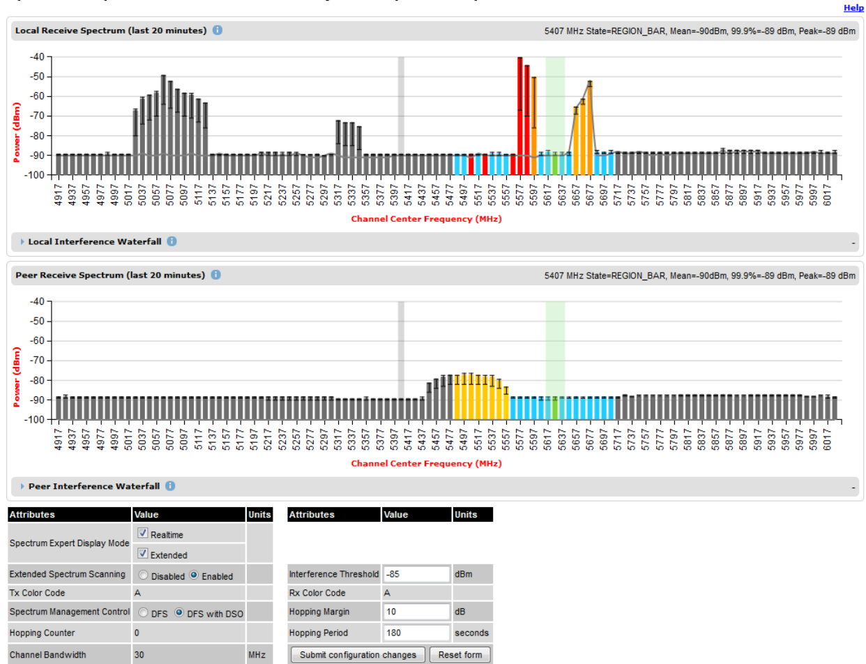
Figure 198 Spectrum Expert page with radar avoidance – Extended Display
