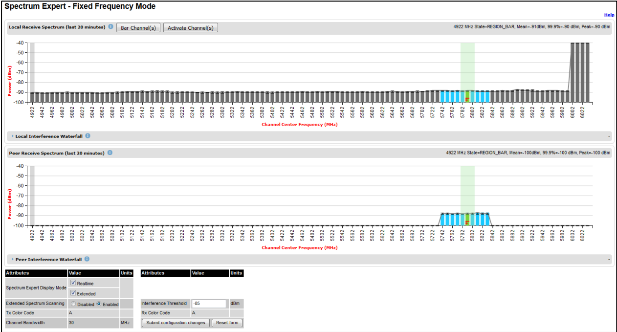
Figure 196 Spectrum Expert page for Fixed Frequency – Extended display mode
