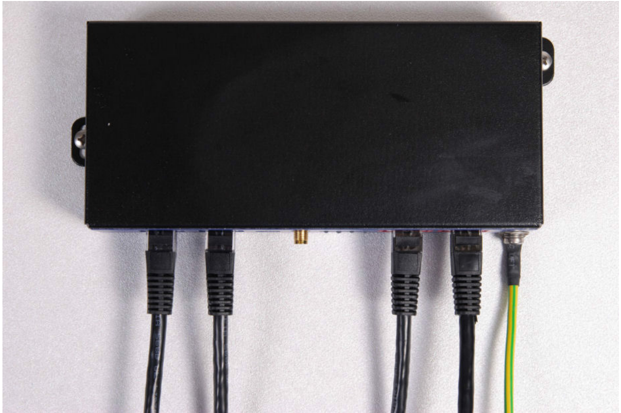
Figure 110 PTP-SYNC mounted on a wall
